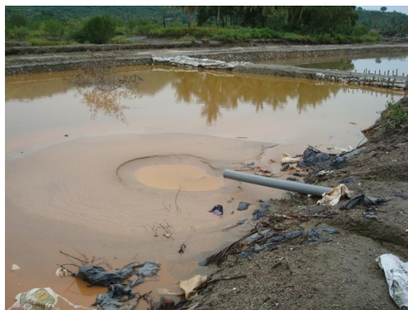
Coastal cyanidation facility in the Sekotong ASGM area. Tailings is discharged into the containment pond which was once used for aquaculture. This pond is open to the sea.
