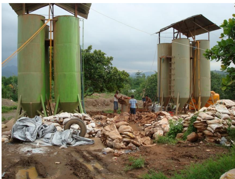
A cyanidation facility on Sumbawa. The bottom photo shows sacks of amalgamation tailings ready for leaching. Spent tailings are discharged into an excavated hole (main photo)
