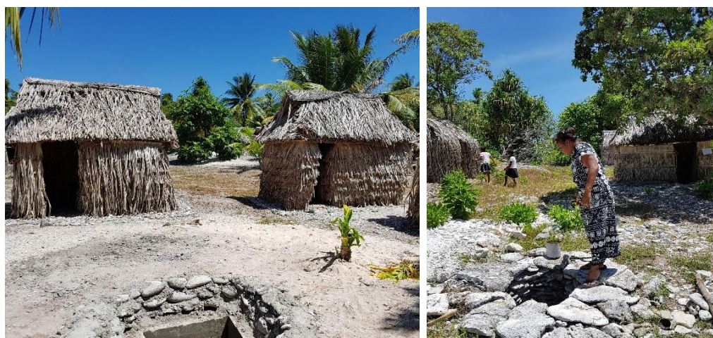
Figure 1 - Toilets built close to unprotected water wells in Aontena JSS (left) and Ueen Abaiang JSS (right)
